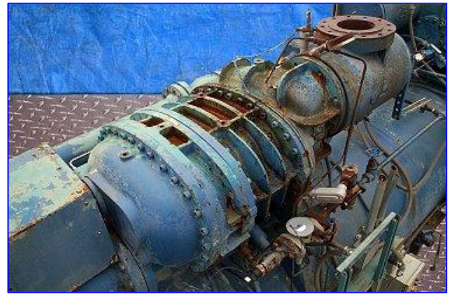
Second Compressor Model: RWB126B, S/N 2512X421, REFRIG NH3, Vol. Ratio-----2.4, Max Speed-----3,600 RPM, Max Pressure--300 PSIG.
