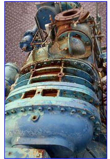
Second Compressor Model: RWB126B, S/N 2512X421, REFRIG NH3, Vol. Ratio-----2.4, Max Speed-----3,600 RPM, Max Pressure--300 PSIG.
