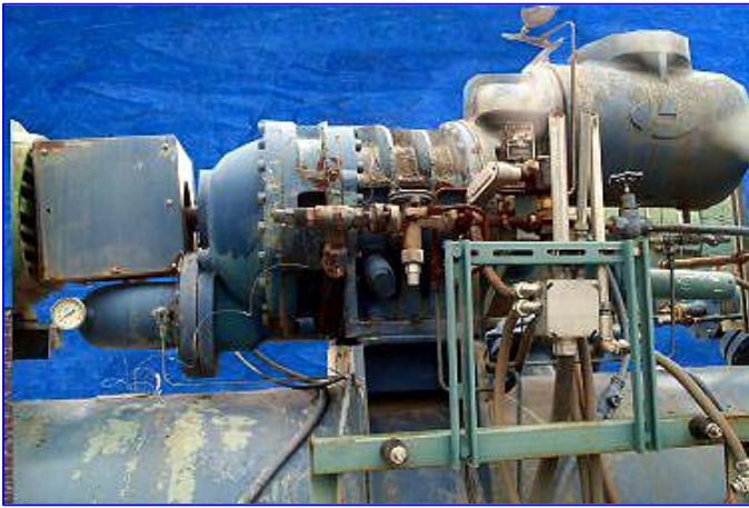
Second Compressor Model: RWB126B, S/N 2512X421, REFRIG NH3, Vol. Ratio-----2.4, Max Speed-----3,600 RPM, Max Pressure--300 PSIG.
