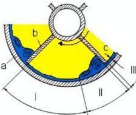
Fig. 1: a) inner shell b) rotor blade c) gap between rotor and inner shell I) film zone II) bow wave III) gap zone
