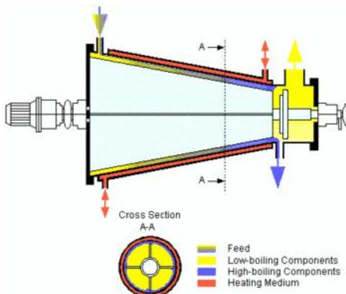
Fig. 4: Horizontal conical design type "Sako KH"
