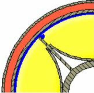
Fig. 5: Cross-section of Thin Film Evaporator Type "LUWA"
