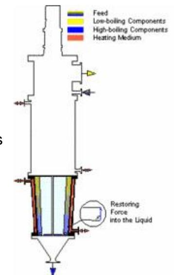
Fig. 3: Vertical conical design type "Sako KV"
