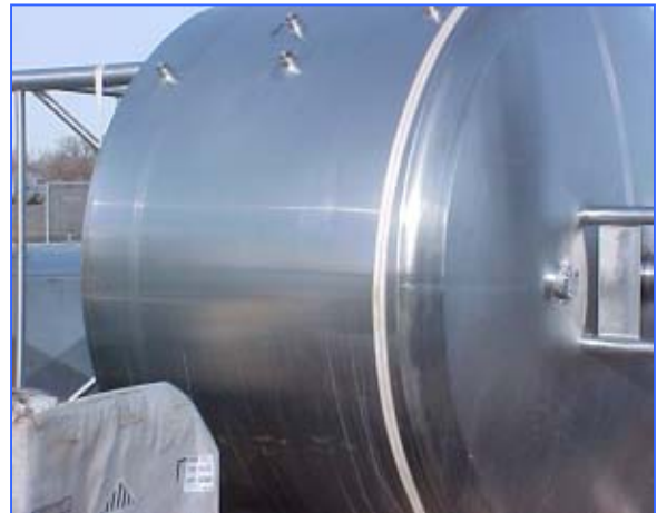
1996, DCI 1500-gallon processor, stainless steel, dome top, cone bottom, serial no 94-D-49834-B, with scrape surface agitator.
