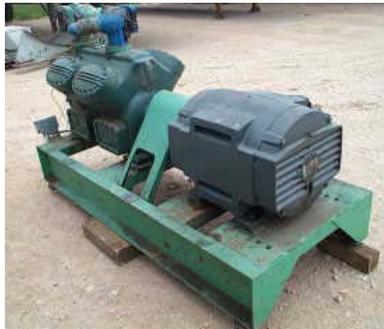
Carrier Air Conditioning Co. compressor model no. 5H80-8129 serial no. 4049488, 76 inch x 32 inch.
