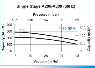
Performance curves are based on dry air at 68°F (20°C), 60°F (15°C) seal water, and 29.92 inches of mercury (760 torr) barometric pressure.
