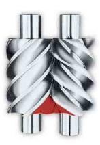
Discharge Phase — At a point determined by the designed "built-in" compressor volume ratio (V), the discharge port is uncovered and the compressed gas is discharged by further meshing of the male and female interlobe space. While the meshing point of a pair of lobes is moving axially, the next charge is being drawn into the unmeshed portion and the working phase of the compressor cycle are repeated.
