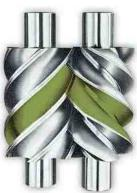
Compression Phase — As rotation continues, the gas in the interlobe space is carried around the circumference of the compressor housing. Further rotation meshes male and female lobes thus reducing interlobe volume. Positive displacement compression continues in the direction of the discharge port.
