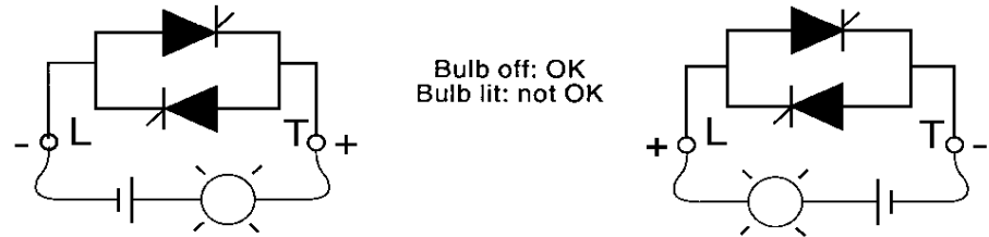
Figure 37 Checking Thyristors
