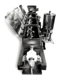
Groen Continuous Screw Blender and Coater. Model CSB. Is idea for coating popcorn and can be used to process a variety of products requiring continuous mixing and uniform coating. The Model CSB can be sized to meet your product residence time and throughput requirements and is equipped with an appropriate flight screw for proper particulate mixing and coating action. The trough shaped shell is normally fitted with a high pressure jacket, designed for either heating or cooling applications.
