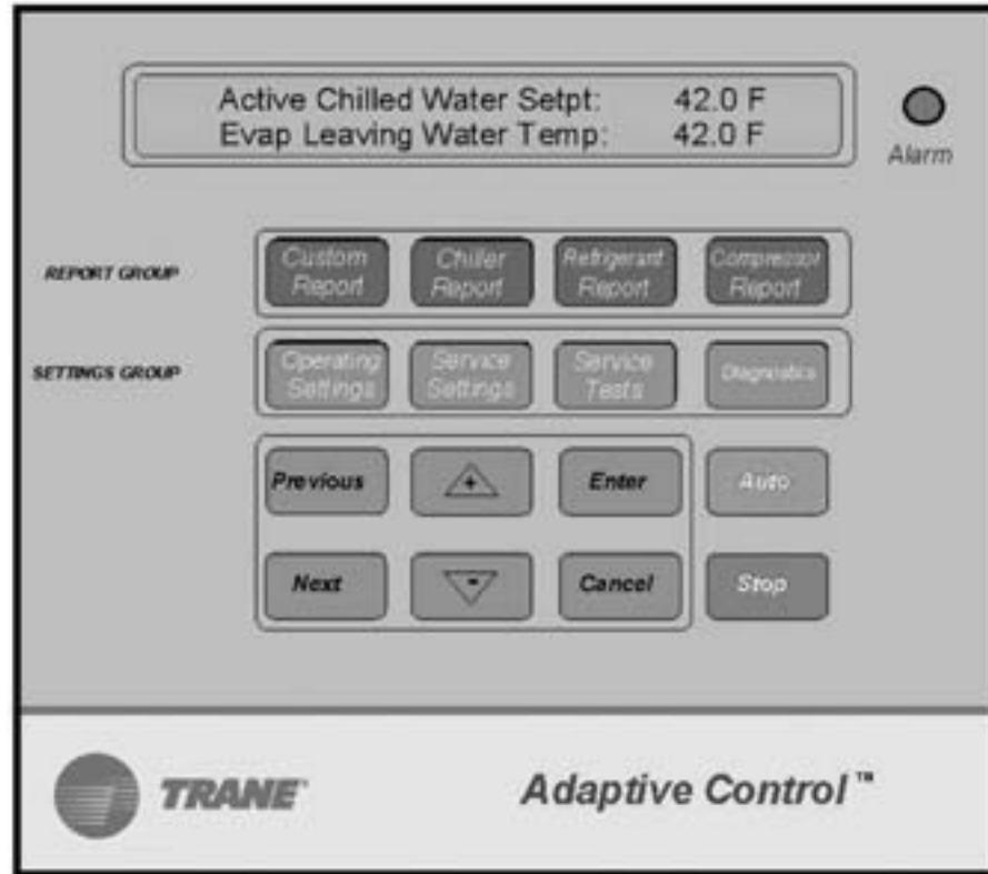
Figure 35 Operator Interface Adaptive Control
