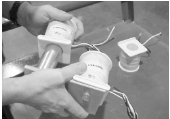
Fig. 29 – Install new coils on cores
