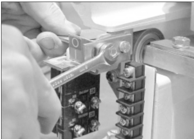
Fig. 30 – Remove the two mounting screws securing the contact assembly to bearing retainer
