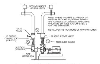
Fig. 4 - Typical Installation - Vertical Piping
