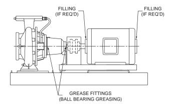
Fig. 5 - Lubrication Points
