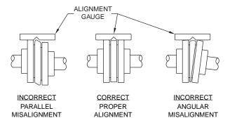
Fig. 2 - Coupling Alignment
