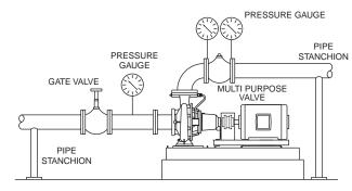
Fig. 3 - Typical Installation - Horizontal Piping
