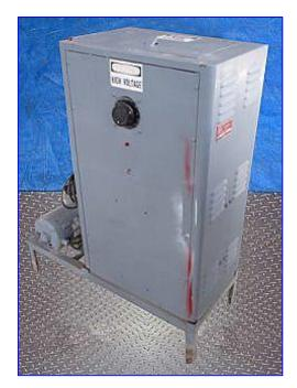
Ozone Sterilization System, Hess Machine Company, Ephrata-PA, Model H-50, S/N I27587-R, with self contained air compressor 3/4 hp 115/230 volts 1,725 rpm, 115 volts transformer.
