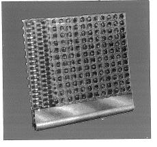
**4.** This leaf is our standard construction for sluicing filters. The leaf comprises a keyhole frame with a tubular slit drainage member welded to the frame. Polypropylene netting is attached to the drainage member and the whole leaf covered with a fabric bag (not shown for clarity).
