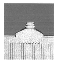
**7.** This shows nozzle outlet area of typical polypropylene leaf. This leaf, which is only used on a sluicing filter, requires a fabric bag while in operation. The grade of polypropylene used is the best available and is inert to most chemicals. There is, however, a temperature limitation of 194° F (90° C).
