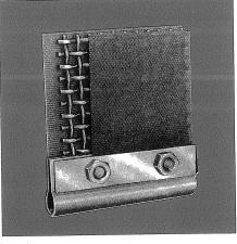
**2. and 3.** Same as No. 1 except that No. 2 has riveted construction and No. 3 has bolted construction to facilitate screen replacement.
