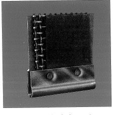
1. This construction is the most economical metalic leaf manufactured by FSD: It has a keyhole frame, 4 X 4 mesh drainage rnember with 24 X 110 P.D.W. screen. The whole system is spotwelded together.
