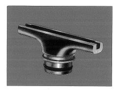
**9.** Typical outlet nozzle. Standard material is 316 stainless steel which is investment cast then machined to very close tolerances. A positive seal is obtained by the use of an "o" ring.
