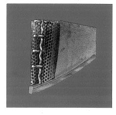
6. A circular leaf of 7 ply construction developed for the brewing industry. Using a bar frame with heavy duty 1 X 1 drainage member, perforated plate and 16 mesh interrnediate members with a 24 X 128 surface screen (60 micron nom.). The surface screen is laser welded to the bar frame by a method developed by FSD (patent applied for)
