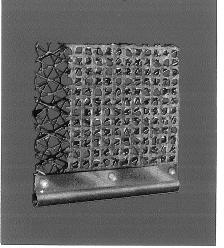
**8.** Titanium leaf – this construction is the choice for highly corrosive applications. It is strong, but light in weight. The design incorporates a keyhole frame with a 2 x 1 and two  $1^{1/4} \times 1^{1/2}$  expanded metal screens for drainage. A polypropylene netting is then attached to the screen prior to a bag being fitted.
