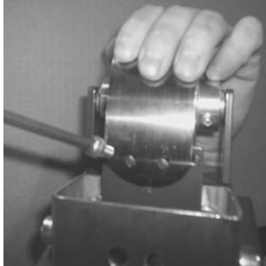
Figure 15: Pivot spring in place to line up with spring/actuator bracket and reinstall hardware.
