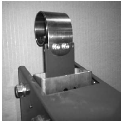
Figure 8: Slide head up to expose spring mount hardware. Then lock in place using lock knob on the side of head weldment.
