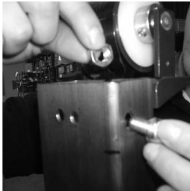
Figure 16: Reinstall head stop hardware in mast assembly. (1) near side (1) far side
