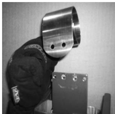
Figure 10: Remove spring from spring/actuator bracket.
