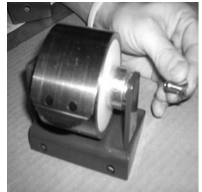
Figure 13: Insert constant force spring assembly into spring bracket. The spring should be facing the rear of the bracket as shown.
