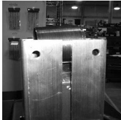
Figure 7: Slide head upward until spring is forced outside of mast.
