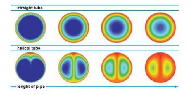
The figures above show the heat distribution of a fluid flowing in a straight tube and a curved tube in relation to tube length. The wall temperature is 100°C, the tube diameter is 0.025 meters and the rate of flow is 1 meter/sec. The situation is shown after 1 meter, 30 meters, 100 meters and 200 meters. Blue, green, yellow and red indicate the rising temperature.
