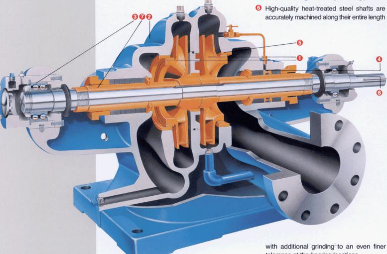
quiet operation. Impellers are firmly keyed and locked to an accurately finished oversized shaft to absorb all shock loads.
