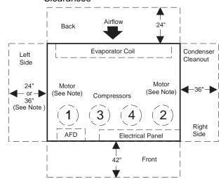
**Note:** (1) 36 inches is required if piping connections are left hand or fan discharge is back.
