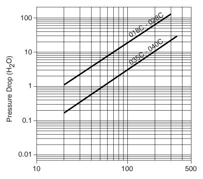
Condenser Flow Rate (gpm)
