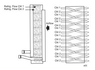
All evaporator coils are interlaced circuiting, keeping the full face of the coil active to eliminate air temperature stratification. For optimum part load performance, all three and four circuit evaporator coils are circuited for both interlaced and row control. Compressor staging is sequenced to take maximum advantage of available coil surface.
