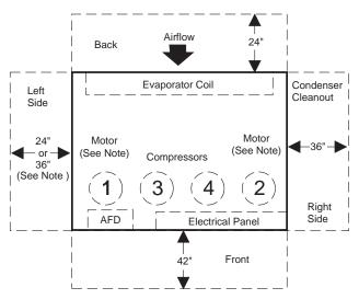
**Note:** 36 inches are required if water and condensate drain connections are left-hand, or fan discharge arrangement is back.
