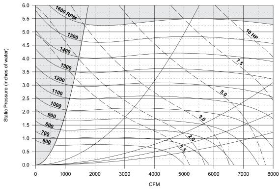
Figure 23. SWT018C, 15"x15" Fan Without Variable Inlet Vanes
