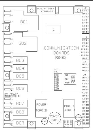
Analog Inputs Terminal Block (J8)
