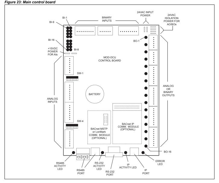
**LED Operational Check Period.** When power is applied to the MCB or when the MCB is reset, an operational test of the 16 Binary Input LEDs (in the upper left corner) and the four miscellaneous status LEDs (at the bottom of the MCB) is performed, which provides a visual check of the operational status of the LEDs. The following LED sequence should occur:
