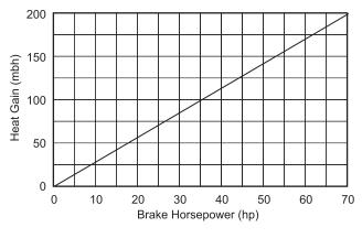
Fan Temperature rise = (Fan Heat (Mbh))(1.085 x Fan cfm)
