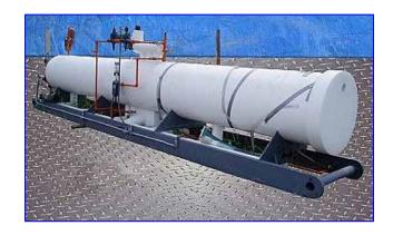
This unit Model: WC-125HV-2000HSS. S/N: WC-992-685 was built new in 1985 and its designed capacity was 85 ton at 20 ° F. ammonia temp at the heat exchanger.
