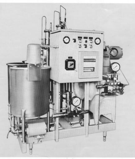
■ **PRODUCES STERILE PRODUCT**—Unitherm "No-Bac" processing protects product from contamination during processing ... sealed from input to output.
