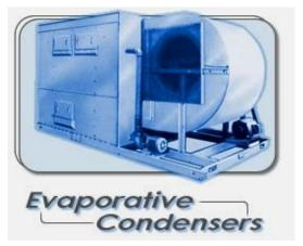
The Recold JC series is a forced draft, centrifugal fan, counterflow Evaporative Condenser. The unit is of low profile design with a single fan mounted on the end of the unit for convenient access by service personnel. The unit ships completely factory assembled with optional accessories factory installed unless specified otherwise.
