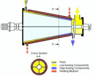
Fig. 4: Horizontal conical design type "Sako KH"
