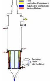
Fig. 3: Vertical conical design type "Sako KV"
