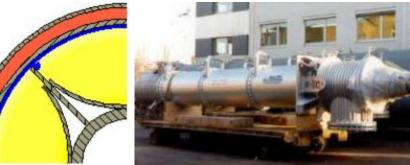
Fig. 5: Cross-section of Fig. 6: Thin Film Evaporator Type Thin Film Evaporator "LUWA" Type "LUWA"
