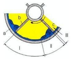
Fig. 1: a) inner shell b) rotor blade c) gap between rotor and inner shell I) film zone II) bow wave III) gap zone
