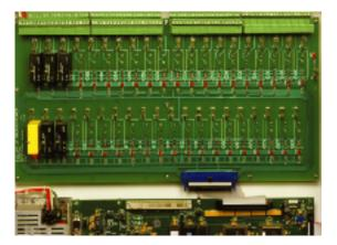
Two screw type terminals are provided for each connection point to allow for more field wiring connections to be made without additional external terminals.
