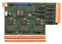
*Communications:* The Micro III supports the high-speed peer-to-peer ComMENT network interface with easily wired screw terminal connections. The board also supports a 9-pin RS-232 or a 5-terminal screw-type connector RS-422 serial interface port. The RS-232/422 serial interface is currently used for program downloads to flash memory.
