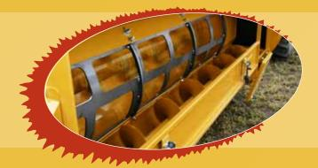
**Two-stage Bale Loader:** Haybuster's HD two stage bale loader not only loads bales but also carries a second bale to improve feeding/bedding/mulching efficiency.
