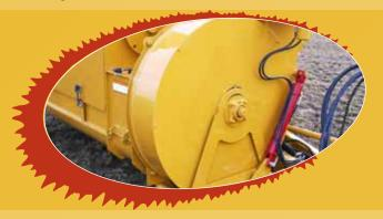
**Bale Chamber/Slug Bar:** The Bale chamber with the three chain slat conveyor (live floor) is built heavier and higher to withstand the weight and size of today's larger bales. The 9 heavy-duty adjustable slug bars allow for wide range of adjustments for various products. Ten additional stationary slug bars can be added for more even feeding and a finer cut.
