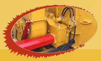
**Fan:** The new fan design is welded on a HD 2 inch shaft for improved fan output. The fan housing and discharge chute is lined with AR 400 high abrasion steel for long life and improved performance. Both horizontal and vertical articulation is accomplished by hydraulics controlled from the tractor cab with a joystick control.
