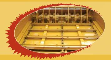
**Access Door/Screens:** The large access door allows easy accessibility to the flail tube, screens and transition auger. Switching from fan discharge to conveyor discharge is also accomplished here, and only takes a few minutes to do the conversion. Screens are available in 2", 3" and 4" round as well as  $4\frac{1}{2}$ " x 9" and  $6\frac{1}{2}$ " x 9"
