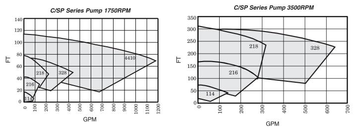
Note! Alfa Laval does not recommend using the C/SP 4410 pump with 3500RPM motors
