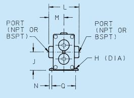
NOTES: 1. SUCTION AND DISCHARGE PORTS ARE DEPENDENT UPON ROTATION. 2. BEARING FLUSH PLUGS (.12 N.P.T.) ARE OPTIONAL. 3. ALL DIMENSIONS ARE IN INCHES.
