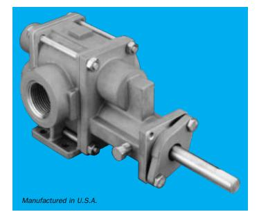
This self-priming, external spur gear pump has 1-inch ports and will deliver flows up to 22gpm. Maximum rated differential pressure for the pump is 100 psi. Designed for simplified maintenance, the pump may be quickly disassembled without the need to break piping connections. The G8 is designed for continuous duty industrial applications with clear, non-abrasive fluids.
