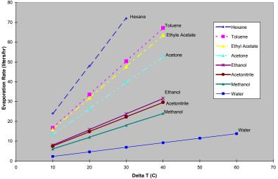
The capacity of the ProTherm 50 depends on the operating conditions and solvent involved.
