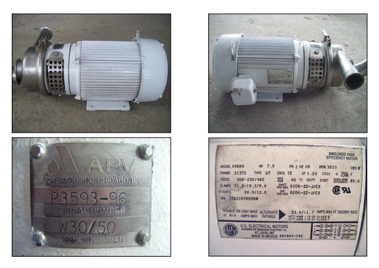
(1) APV Centrifugal Pump: Model no. W30/50. Serial no. P3590-96. U.S. Electrical motor: 3 hp, 1750 rpm, 230/460 V, 8.8/4.4 A, 60 Hz, 3 phase. Inlets: (1) 3 in. s-line. Outlet: (1) 2-1/2 in. S-line. Overall dimensions: 1 ft. 9-3/8 in. L. x 1 ft. <sup>3</sup>/<sub>4</sub> in. W. x 1 ft. 2 in. H.
