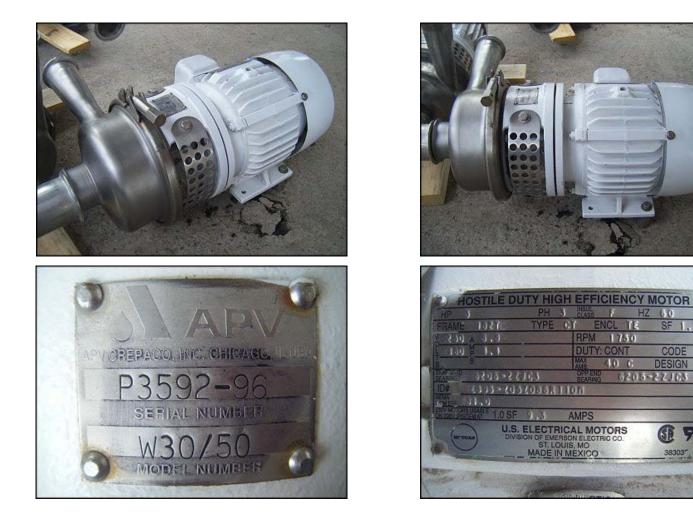
(1) APV Centrifugal pump: Model no. W30/50. Serial no. P3593-96. U.S. Electrical motor: 7.5 hp, 3510 rpm, 208-230/460 V, 24.0/12.0 A, 60 Hz, 3 phase. Inlets :( 1) 3 in. S-line. Outlet: (1) 2-1/2 in. S-line. Overall dimensions: 1 ft. 1 in. L. x 1 ft. 2-1/2 in. W. x 1 ft. 2-3/4 in. H.
