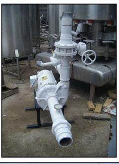
HZ-60 CAT NO- M330 50 MODEL-1K254TF9X7008AA L HP-20 20 FR-254JM PH-3 TYPE- TOX RPM-3470 2910 AMB-40 °C INS-B. DUTY-CONT. VOLT-230/460 230/469 DES-B FLA-47/23.5 41.8/20.9 FLEF 88.5 FLPF 90.4 SF-1.15 1.0 HIGH VOLTAGE OW VOLTAGE SFA-CODE-G ENC. DP TS 1 77 . .... PE BRG- 208 543960 09 OPE BRG- 207 090194
