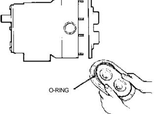
4. Remove rotor retaining nuts. Use the special wrench supplied with pump and hit it sharply with a soft hammer to loosen nuts.
