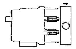
**CAUTION:** Body must be reassembled on bearing housing from which it was removed. Both are identified with same serial number.
