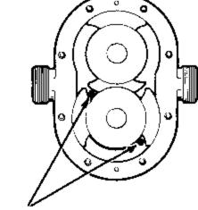
5. Orient rotors perpendicular to each other and remove rotor with both wings exposed first. Handle rotors with care to avoid knicks and scratches. If it is stuck tight, use a gear puller or hardwood lever behind rotor hub to force it off spline.
