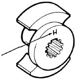
**NOTE:** All hot clearance rotors are identified with a etched letter "H" on rotor hub.
