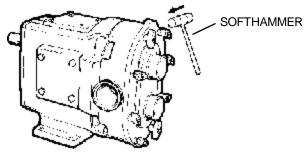
3. Remove cover. If it is stuck, loosen it with a soft hammer. Remove and discard cover "O" ring.
