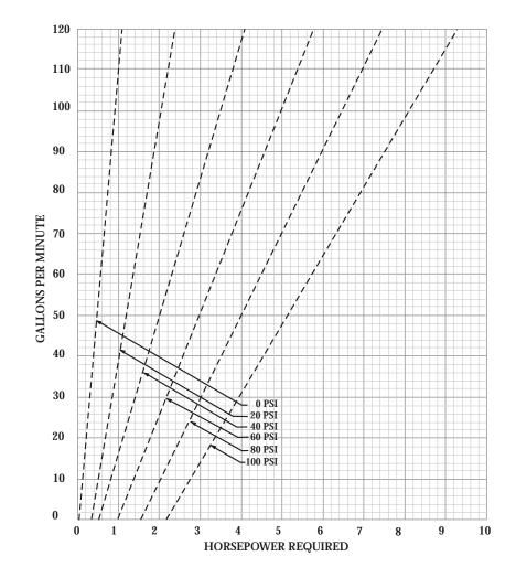
Note: This graph is predicated upon liquids of the viscosity and specific gravity of water and milk at  $100^{\circ}$ F ( $34^{\circ}$ C). The horsepower ratings are actual brake horsepower. This graph applies to polymer coated rotors only.
