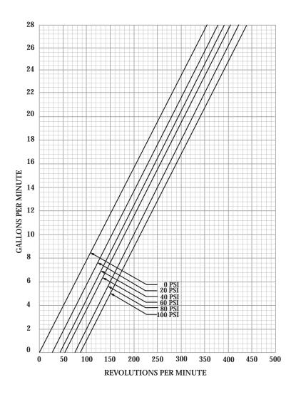
Note: This graph is predicated upon liquids of the viscosity and specific gravity of water and milk at  $100^{\circ}$ F ( $34^{\circ}$ C). The horsepower ratings are actual brake horsepower. This graph applies to polymer coated rotors only.
