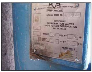
1994 Refrigeration Valves & Systems Vertical Receiver- 18 Gallon. S/N: 94407. Nat'l Bd: 6754. Inside straight-wall dimensions: 1 ft. 1 in. dia. x 2 ft. 8 in. H. MAWP: 250 psi @ 300°F. MDMT: -20°F @ 250 psi. Inlets: (1) 1/2 in. dia. port, (1) 1 in. dia. port. Outlets: (1) 1/2 in. dia. port, (1) 1 in. dia. drain port, (2) 1 in. dia. ports (relief) (1) 1-1/2 in. dia. port. Overall dimensions: 3 ft. 7 in. L x 3 ft. 4 in. W x 6 ft. 4 in. H.
