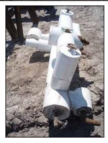
Hansen Technologies Hermetic Centrifugal Pump. Model: 2003. Order No: 411001011/031-01. Type: CAM2/3. Maximum capacity: 52.7 gpm @ 105 tdh. Minimum capacity: 5.27 gpm @ 177 tdh. Impeller diameter: 4.48 in. Nominal pressure: 362 psi. AGX Motor, 6.3 hp (4.7 kW), 3380 rpm, 440 V, 7.5 amps, 60 Hz, 3 phase. Inlets: (1) 1-1/2 in. dia. flanged port. Outlets: (1) 1 in. dia. flanged port. Overall dimensions: 2 ft. L x 9 in. W x 10 in. H.
