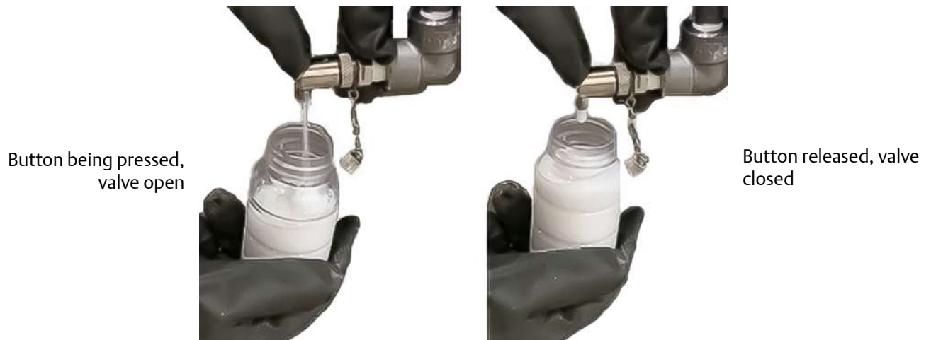
Figure 5-5. Operating the Oil Sampling Valve
