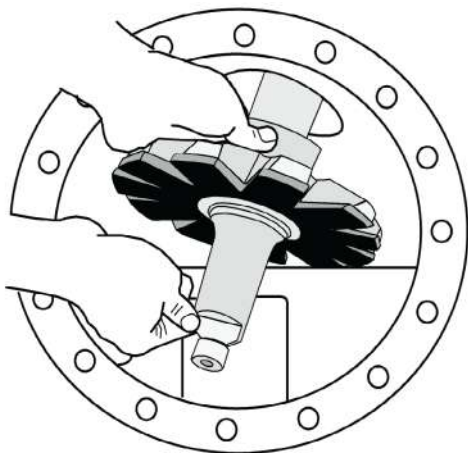
Figure 5-47. Gaterotor Assembly Removal
