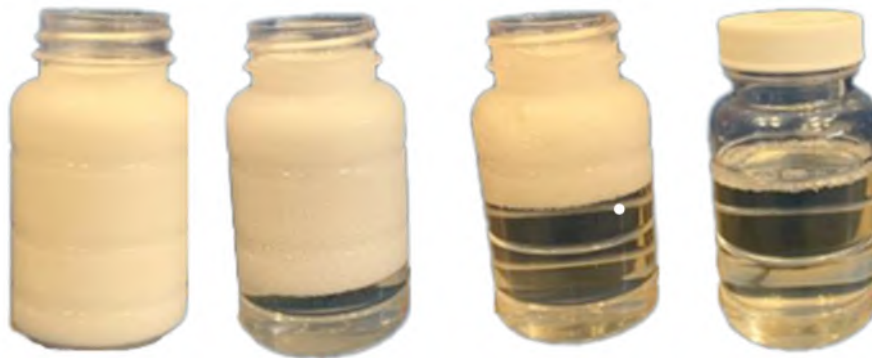
Figure 5-6. Stages of the Oil Sample Taking Process
