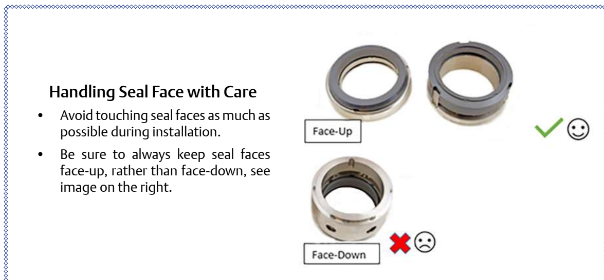
Figure 5-59. Handling Seal Face with Care
