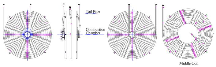
Figure 1: Heat Exchanger Configuration
