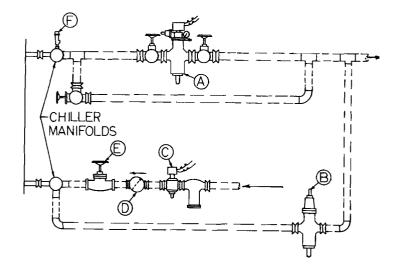
**Control Includes**: Combination suction pressure regulator stop valve with pressure gauge; relief (defrost) valve; liquid solenoid valve with strainer; check valve; hand expansion valve; manifold relief valve; full suction by-pass.
