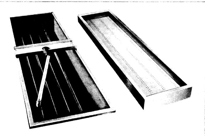
Above is top view of a four-section Closed Type Chilled Water Unit with covers and distributing trough removed. Trough fits under feed pipe, which is also shown. Cross piece permits dividing top covers into two sections, and opening in it enables feeding unit from top - by gravity if desired. Distributing trough for four sections is shown above. Note holes which evenly distribute liquid over both sides of each section.
