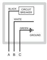
Fig. 17: Wiring Connections
