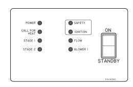
Fig. 28: External LED Indicator Decal
