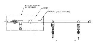
Fig. 15: Gas Supply Connection
