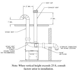
Fig. 27: Direct Vent - Vertical
