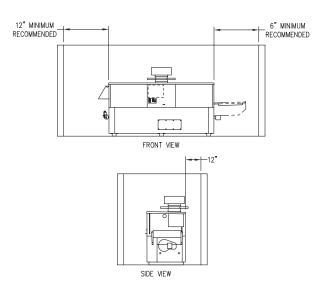
Fig. 7: Minimum Clearances from Combustible Surfaces – Outdoor Installations
