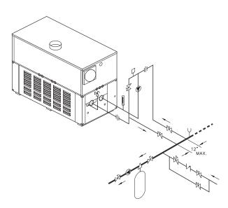
Fig. 10: Single Heater - Low-Temperature (Heat Pump) Application with Primary/Secondary Piping
