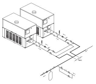
Fig. 11: Dual Heaters (Reverse/Return) with Primary/Secondary Piping
