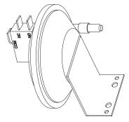
Fig. 36: Blocked Vent Switch
