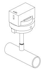
Fig. 34: High/Low Gas Pressure Switch
