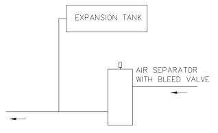
Fig. 9: Air-Separation/Expansion Tank
