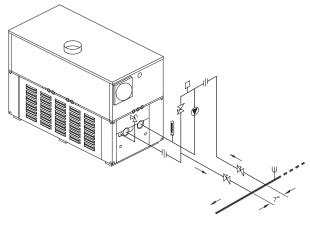
Fig. 13: Single Pool Heater Application
