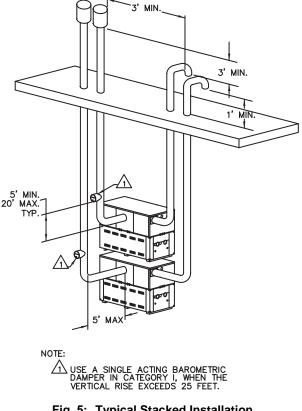
Fig. 5: Typical Stacked Installation
