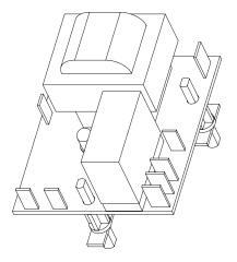
Fig. 33: Low Water Cut-Off
