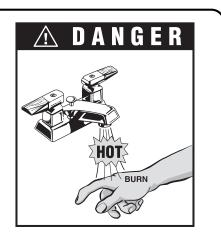
Water temperature over 125°F can cause instant severe burns or death from scalds.
