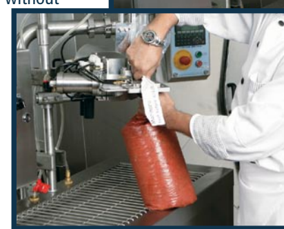
Station-mounted clipper for sealing, attaching label and trimming casing
