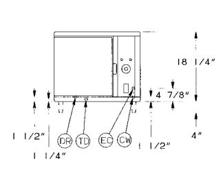
INCOMING WATER HARDNESS SHOULD NOT EXCEED 2 O GRAINS AND PH NOT TO EXCEED 7.5 FAILURE DUE TO INADEQUATE WATER QUALITY IS NOT COVERED UNDER MANUFACTURERS WARRANTY.
