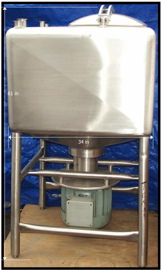
Breddo Liquifier Model LDD-100 Gallon, Serial Unknown, single shell, 20 HP, 1745 RPM, 230/460 V-3 phase-60Hz, 18 in manway, 34 in L x 34 in W x 61 in H, p-102-B.75a
