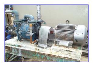
Lincoln Motor, S/N 2300608. 15 hp, 3 phase, 230/460 volt, 40/20 amps, 60 Hz, 1,750 rpm. Pump does not have any information.
