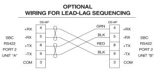
USE BELDEN #8777 OR EQUAL (3 TWISTED PAIRS) COLOR CODING SHOWN IS BELDEN #8777 RS 422 WIRING SHALL BE SEPARATE FROM ALL OTHER WIRING
