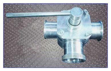
Working Principle: A polytetrafluoroethylene (PTFE) shutter is operated by means of a handle or an actuator. A spring washer system presses the shutter against the internal cylindrical surface of the valve body, ensuring a tight seal.
