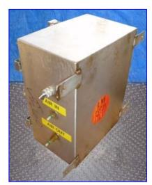
Honeywell Control Panel. Honeywell control box. 90-250 V, 50&60 Hz, 18 VA. Ambient limits:  $32^{\circ}F$  to  $131^{\circ}F$ . Overall dimensions: 10-1/2 in. L x 12 in. W x 18-1/2 in. H.
