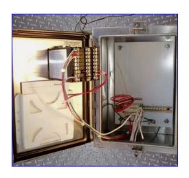
Honeywell Circular Chart Recorder. Model: DR45AT-1100-001-0-000000-0. S/N: 0214Y254457100001. Control requirements: 120/240 VAC, 50&60 Hz, 20 VA, set 120 VAC, operating temp: 32°F to 131°F. Overall dimensions: 41 in. L x 12 in. W x 48 in. H.
