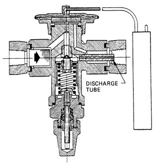
TYPE A THERMAL EXPANSION VALVE (20-100 TONS) R-717
