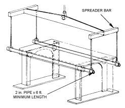
FIG. 1 - RECOMMENDED LIFTING METHOD
