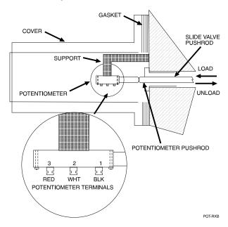
**5. ADJUSTMENT** must be made with the slide valve fully unloaded and the compressor running. The Operating display at this time should indicate a slide valve position of 0%. If the display is greater than 0%, adjust potentiometer POT #4 on the SBC until 0% is indicated. If 0% is not attainable, get as close as possible and then proceed to the next step. The adjustments of POT #4 and POT #3 are interactive and POT #3 may require adjustment to allow POT #4 to come into range.
