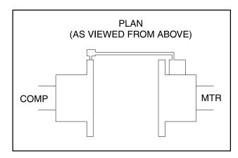
FIG. 5 - DIAL INDICATOR ATTACHED (AT 9 O'CLOCK)
