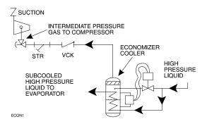
FIG. 1 - SHELL and COIL ECONOMIZER SYSTEM
