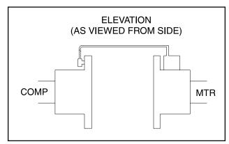
FIG. 2 - DIAL INDICATOR ATTACHED (AT 12 O'CLOCK)
