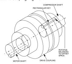
FIG. 3 - COUPLING/SHAFT KEYS INSTALLATION
