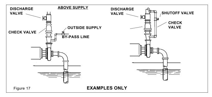
The pump will not self prime if liquid supply is **below** pump level. (Figure 17)
