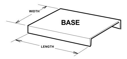
Base plates (OPTIONAL) are provided in three widths and five lengths (depending on motor frame and pump model.)
