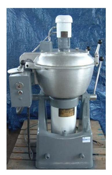
For high speed cutting, mixing, and blending. Has a glass, flip-top manhole 13"x4" and a flip top lid with latch for container portion. Large motor on bottom, small motor on top. No inlets or outlets; emptied and filled by pouring. Has control box on one side and a handle for pouring on other side. Inside dimensions: 19 1/2"diameter, 10 1/2"H. Outside dimensions: 25"W, 29 1/2"L, 51 1/2"H.
