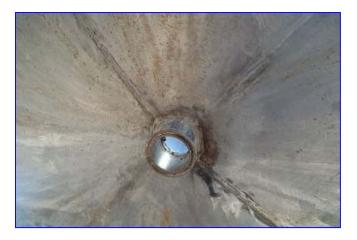
Tank Stainless Steel 300 gallon with Lightning mixer. Slopped bottom with 2 in. outlet in center. Sitting on 4 legs, 25 in. H. March motor, model TE-MDX-MT-3, 115/230 volt, 60-50 hz, 3,400-2,800 rpm, 40c amb-cont. This tank was used for zerolux, benzyl peroxide. Overall dimensions 69 in. L x 44 in. W x 100 in. H.
