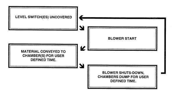
VCL Chamber Level Switches are normally closed, therefore, when material is covering the Level Switch the system is ready and waiting with available material. As the Level Switch is uncovered the blower begins to *load* (material is *vacuum conveyed* to the selected VCL Material Chamber(s)) for the user specified load time (function 132/142). After the specified load time the system then *dumps* the material; also for a user specified dump time (function 133/143).
