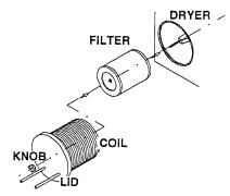
installation of a cooling coil in the return air line. The return air temperature to the dryer should be regulated to approximately 125° F. (50° C.)
