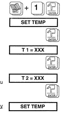
After keying in the selection, press the Enter key and the display will prompt you for the second Setpoint entry: T2 = XXXXXX is the current Setpoint temperature
