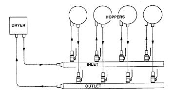
To insure complete flexibility when setting-up a multihopper system a *manifold* may be used. This allows operators to close-off an air inlet on an empty vessel, or completely isolate with minimum delay, a hopper from the system by closing the air inlet and outlet.
