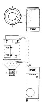
Given air at 200° F. with a -40 dewpoint, the desiccant will only adsorb 4 percent moisture. That same air cooled to 100° F. (36.2° C.) will allow the desiccant to adsorb 14 percent moisture. At 100° F. the desiccant is **3 1/2** times more efficient.
