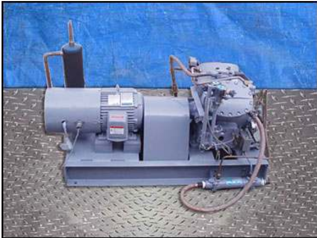
Carlyle Open-Drive Reciprocating Compressor. Model 5F40-149. S/N 2698J01090. Cylinders: 4. Nominal hp: 20. Output: 39.8 cfm @ 1750 rpm. Slightly used. Complete with water cooled heads, external unloaders, auxiliary external oil pump, service valves and mounting frame.
