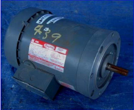
Dayton, 1-½ hp, 3,450/2,850 rpm, 208-220/440 volt, 4.4-4.2/2.1 amps, 60/50 hz, 3 phase, G56C.
