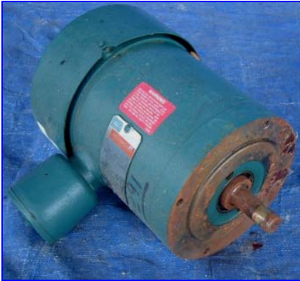
Reliance, 3/4 hp, 1,725 rpm, 208-230/460 volt, 2.8-3.0/1.5 amps, 60 hz, 3 phase, FB 56 C frame.
