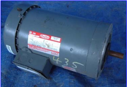
Dayton, 3 hp, 1,725 rpm, 230/460 volt, 9.4/4.7 amps, 60 hz, 3 phase, L56C frame.
