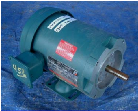
Reliance, 3/4 hp, 1,725 rpm, 230/460 volt, 4.1/2.05 amps, 60 hz, 3 phase, M56C frame.
