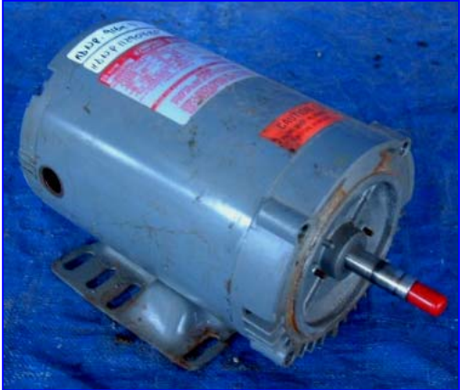
Dayton, 1-½ hp, 3,450 rpm, 115/230 volt, 19.0/9.5 amps, 60 hz, 1 phase, 56J frame.
